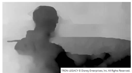
High Strength values add detail, but can cause jagged disparity.
