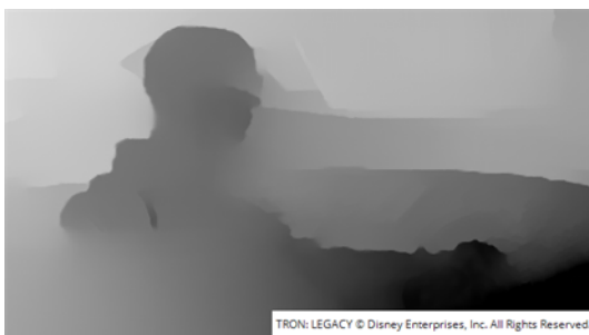
Low Strength values smooth the disparity map, but can miss local detail.
