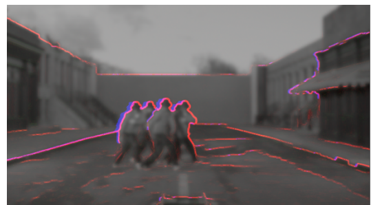
The left view with DisparityReviewGizmo node highlighting any depth changes, alignment changes, and occluded regions.
