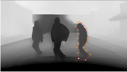
The original left view of the disparity map with a bezier marking the selected area.
