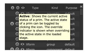
To make searching easier, you can filter your pop up scene graph by searching for keywords, or you can use the new filter types to quickly show only the cameras or materials in a scene and then activate or deactivate them all at a click of a button using the column controls.
